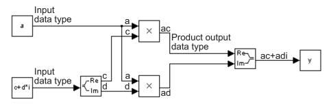
**Complex-Complex Multiplication.** The following diagram shows the multiplication of two complex fixed-point numbers. Note that the output of the multiplication is in the sum data type, which is governed by the fimath SumMode property. The product data type is determined by the fimath ProductMode property:
